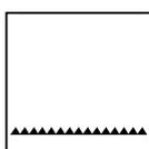
**Non skid.** Safety tile with high-friction surface.
