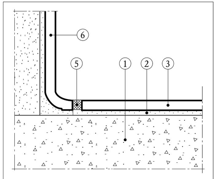
Cross-section through wall/floor with cove skirting tile.
